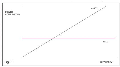
PECL technology offers lower power consumption at higher frequencies, compared to CMOS technology.
